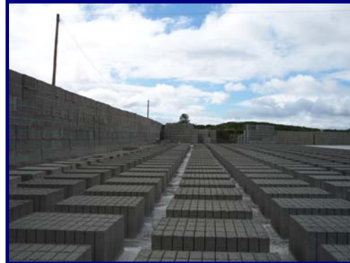
Lightweight (pumice) block production
