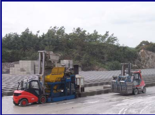
Lightweight (pumice) block production
